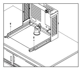
Mount louvered docking assembly using two screws provided.
