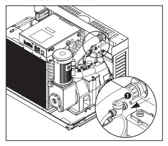
Insert potable water line into valve 1.
