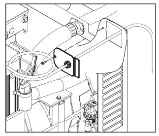
Position plate into opening and secure with supplied screw.
