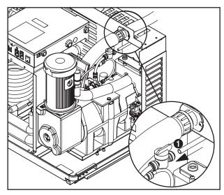
Insert potable water line into valve 1.
