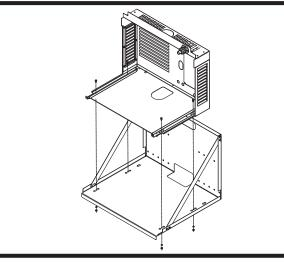
Mount louvered docking assembly to wall bracket accessory
