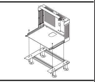
Mount louvered docking assembly to machine stand accessory Install the ice transport tube.
