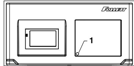
2. Press power switch to turn unit on (**Fig. 5.1**).
