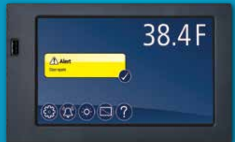
On-screen alarm and event notification. Additional capabilities with battery back-up, including power loss and door open alerts.
