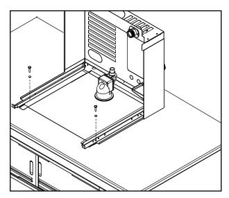
Mount docking assembly using two screws provided.
