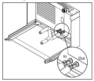
Install ice machine cooling water lines to docking assembly.
