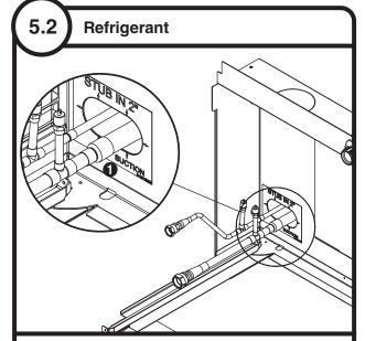
• Braze supplied quick-connect lines onto stub-ins 1.
