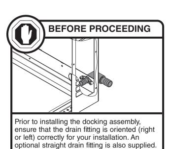
You may need to remove the back panel of the docking assembly in order to re-orient or change the drain fitting. Replace back panel prior to mounting the docking assembly.
