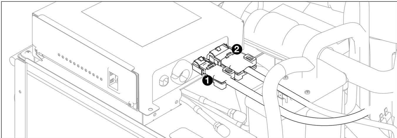
10. On dispensers equipped with water-cooled ice machines, connect condenser water supply and drain lines to condenser fittings on ice machine.
