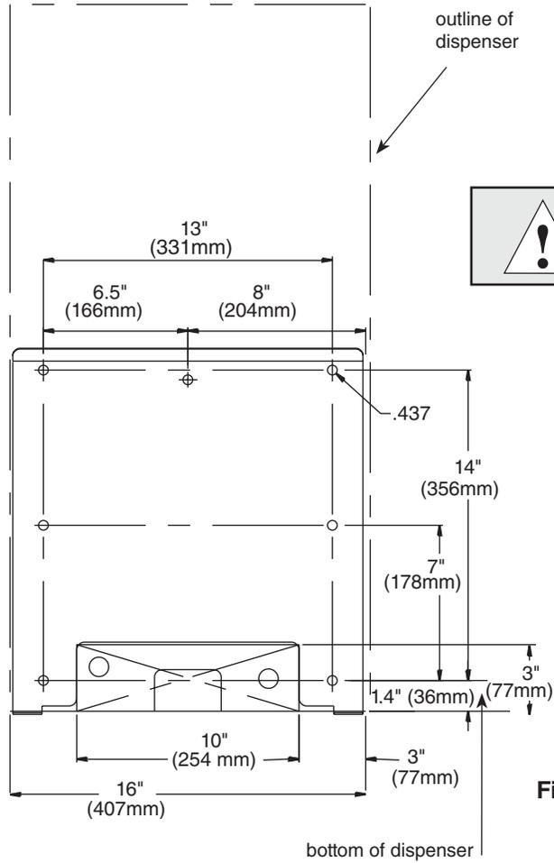
Fig. 7 – Wall mount side view
