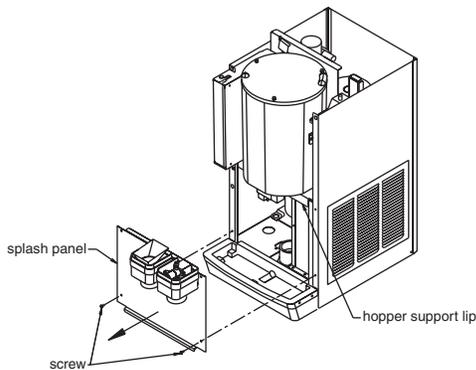
**Splash panel:** Remove 4 screws. Pull out bottom of panel to allow top to slide out from under hopper support lip.
