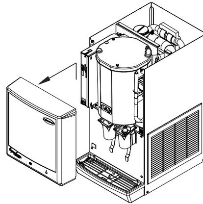
**Front cover:** Pull bottom of cover, then lift cover up and forward to unhook from keyhole slots.
