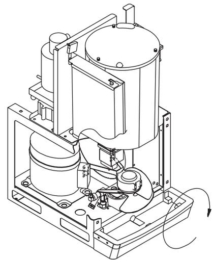
(c) As fan assembly is being pulled toward front, rotate assembly clockwise as shown above.
