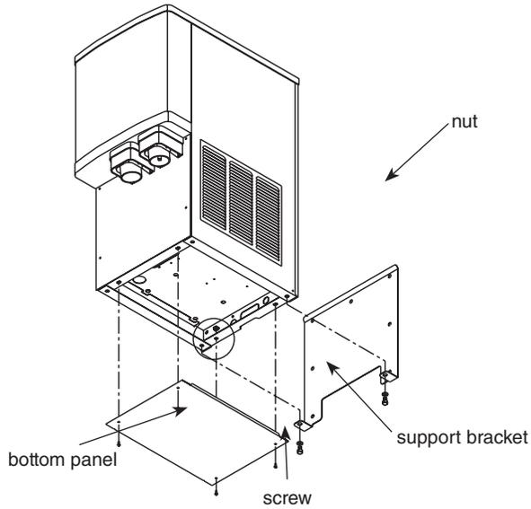
**Fig. 9 – Wall mount bottom view**
