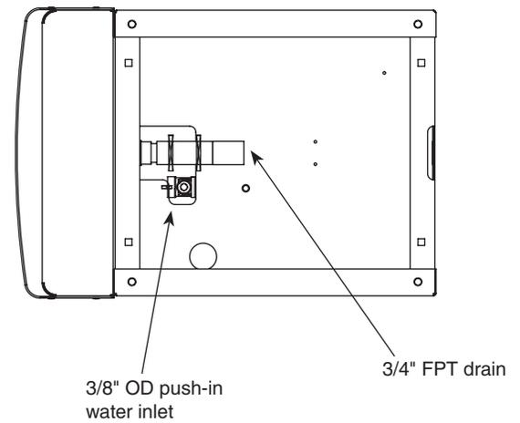
**Fig. 10 – Front view of wall mount bracket, utility location**
