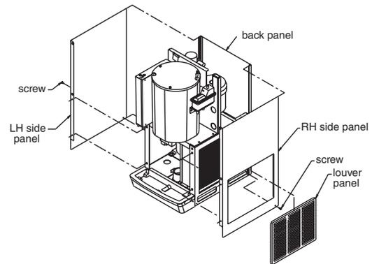
**Side panels:** Remove screw located on lower rear side. Pull side panel toward front of unit and out of back panel. Note: Before removing right hand side, remove side louver panel by lifting up and pulling forward on panel.
