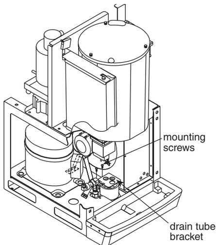
(a) Remove 4 fan mounting screws and 3 drain tubes from bracket.
