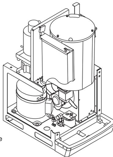
(b) Rotate fan mounting bracket toward back of unit and pull fan assembly toward front of unit.
