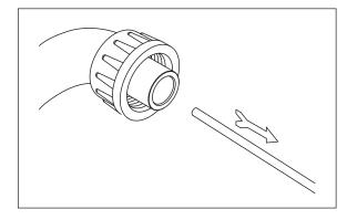
12. Reconnect coupling. Press power switch ON. Ice pushes SaniSponge cleaning sponges through ice transport tube.
