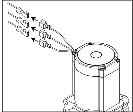
12. Remove gear motor:
