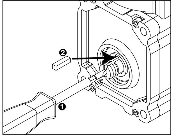
13. Install spacer, ensure that key is captured in slot (**Fig. 25.1**)
