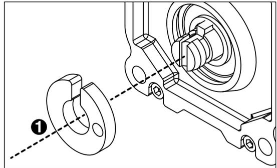
14. Insert screwdriver into groove of auger shaft and pry shaft outwards (**Fig. 26.1**).
