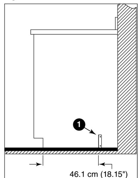
5. Connect water line. Recommended routing (**Fig. 3**) allows easy access to water for cleaning and sanitizing procedure.
